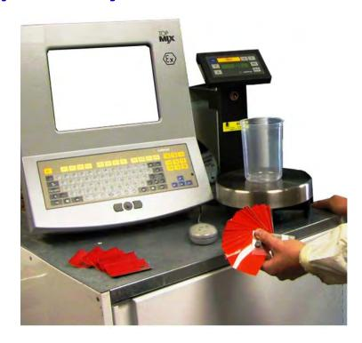
Touch Up Zone uses state of the art computer retrieval software and computer scales to mix precise amounts of each color tint to each formula to ensure proper color match. All mixes are recorded and saved in a database.
