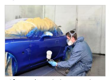
Aftermarket painting operations cannot bake at 350° or apply with Robots. And, most repairs are spot or panel painting.
