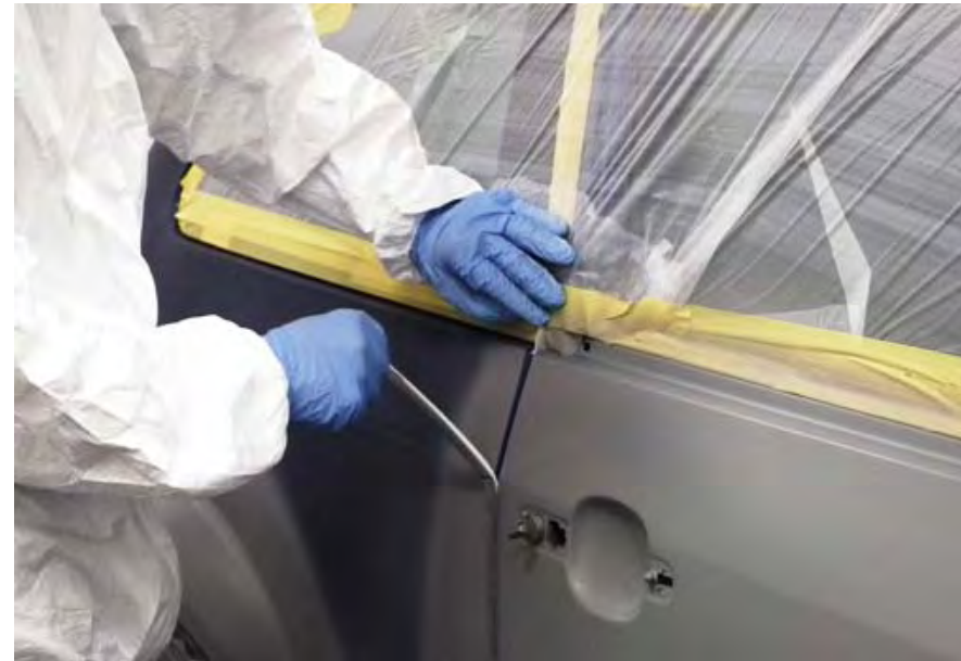
Foam Masking Tape in Cracks & Door Jambs
